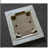
Build the door using lengths of wood and an oblong of plywood. Cut a series of ventilation holes in the plywood. Remember that another piece of plywood will make the inner skin for the door. This will have holes in different places to prevent a direct draught. This
