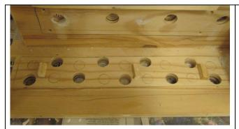
In order to make the side baffles removable for cleaning they were affixed using pegs and holes. A plastic peg set into a small block of wood (see right.) The strategy used here was to place the pegged blocks in place, then to
