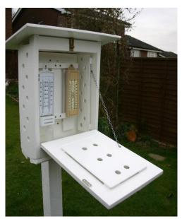
should be mounted on the north facing side of a post so that the bottom of the thermometer is 125cm from floor level.
